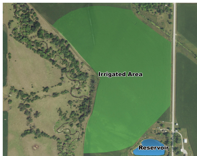
Figure 2. Drainage water recycling site near Story City captures drainage from 20 acres and pumps water from an adjacent stream to irrigate 60 acres.
