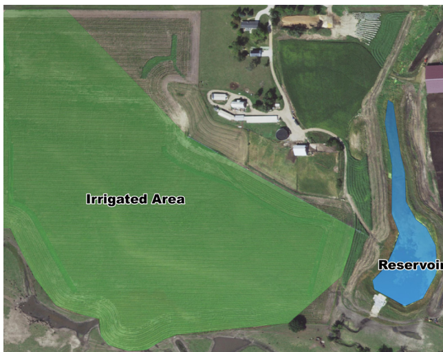
Figure 3. Drainage water recycling site near Lake City captures outflow from an upstream drainage district to irrigate approximately 53 acres.
