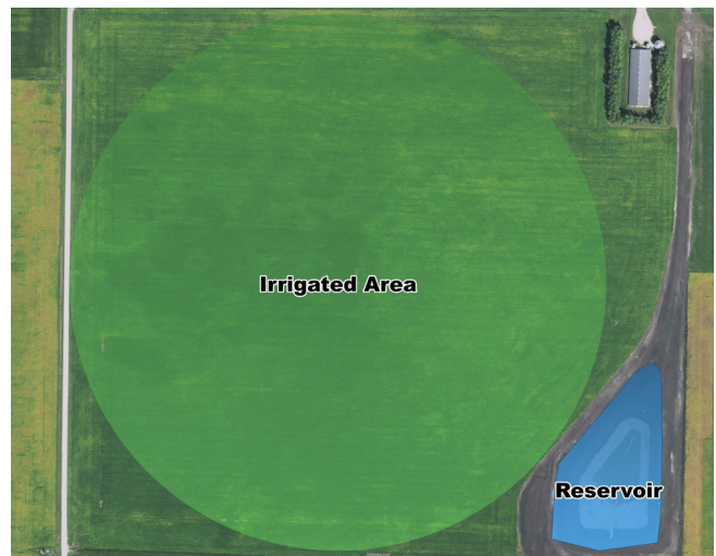
Figure 4. Drainage water recycling site near Dayton pumps water from a county drainage main to irrigate about 106 acres.
